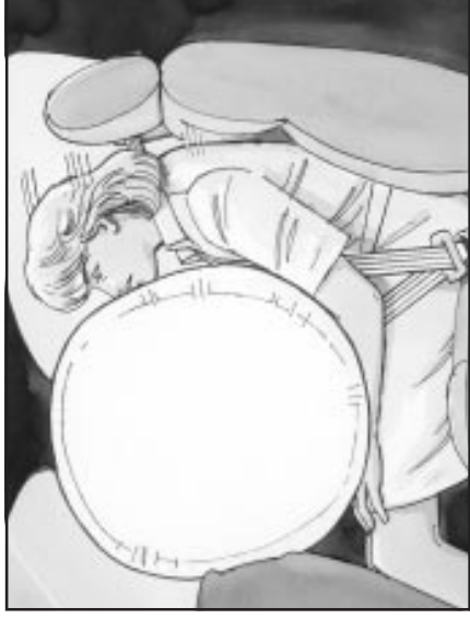
The right front passenger's air bag is in the instrument panel on the passenger's side.
